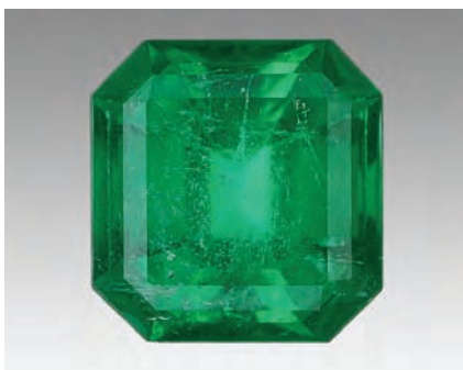
Figure 10. In this 9.96 \times 9.56 \times 7.32 mm polymer-beryl assemblage (left), an inclusion-free region with increasing thickness from the girdle to the culet was easily visible under darkfield illumination at 20 \times magnification (right).
