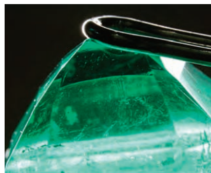
Figure 10. In this 9.96 \times 9.56 \times 7.32 mm polymer-beryl assemblage (left), an inclusion-free region with increasing thickness from the girdle to the culet was easily visible under darkfield illumination at 20 \times magnification (right).
