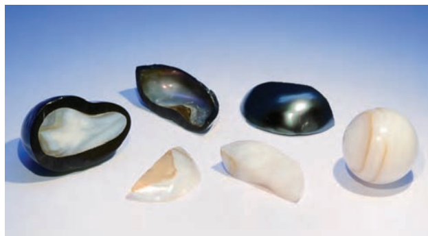
Figure 7. The sawed parts of the specimen are shown next to a classic round nucleus (far right). Both nuclei are similar except for their shape. Photo by O. Segura.
