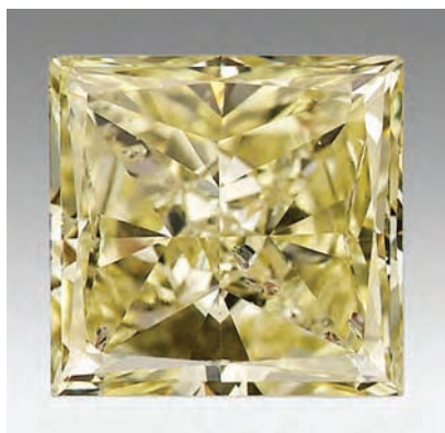
Figure 3. This 2.34 ct Fancy yellow diamond contained a rare contact inclusion pair of diopside and pyrope.
