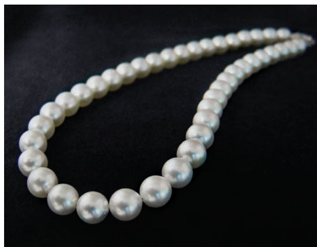
Figure 1. This necklace contains gamma-ray irradiated silver South Sea cultured pearls (12.0–14.0 mm). Electron spin resonance (ESR) spectroscopy proved effective in identifying the gamma irradiation. Photo by Jae Hak Ko.
