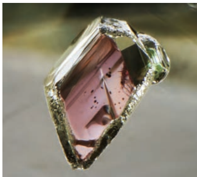
Figure 4. Red and green colors and a reflective interface were observed in the face-up view of the crystal inclusion (left, magnified 75x). Viewing the diamond through the pavilion revealed a small green crystal atop a larger reddish pink crystal (right, magnified 100x). The green crystal was identified as diopside and the reddish pink inclusion as pyrope.
