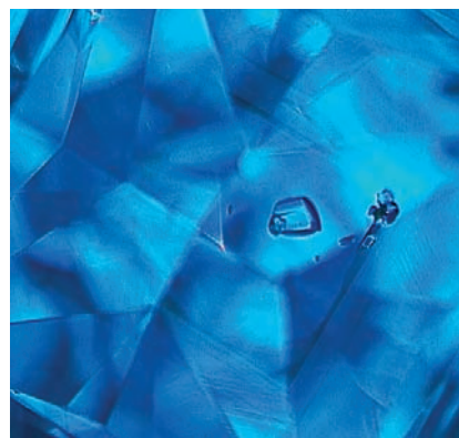
Figure 5. A few isolated prismatic, reddish pink pyrope crystals, the largest reaching the surface, were also visible through the pavilion (left, magnified 75x). The DiamondView image showed that the crystal inclusions formed in different growth zonations (right).
