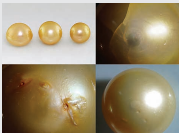
Figure A-1. These three reportedly heat-treated cultured pearls (top left) show various surface characteristics: even light yellow color with no obvious color concentration (top right), patchy yellow color with obvious orange concentrations observed at blemishes (bottom left), and even yellow color with no obvious concentration (bottom right).
