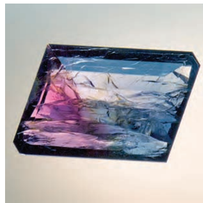
Figure 13. This 14.60 ct gem was identified as a bicolored spinel. Its blue and red zones were caused by the presence of iron and chromium, respectively.
