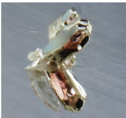
Figure 5. A few isolated prismatic, reddish pink pyrope crystals, the largest reaching the surface, were also visible through the pavilion (left, magnified 75x). The DiamondView image showed that the crystal inclusions formed in different growth zonations (right).
