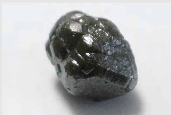
Figure B-1. This 3.11 ct rough carbonado diamond from Sierra Leone is diamagnetic. GIA Collection no. 5914; photo by K. Feral.
