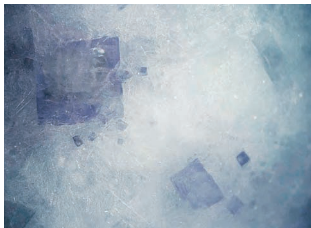
Figure 2. Saturated lavender colors are often associ- ated with a granular texture, sometimes with orthog- onal crystals, as in this Burmese lavender jadeite. The color of these crystals varies noticeably from purplish to bluish when illuminated by directional lighting at various angles. The matrix is mostly whitish. Photo by R. Lu; image width ~12 mm.
